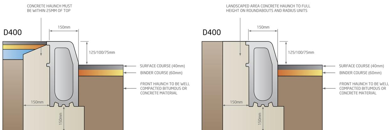
Please note: EN1433 is clear and concise. ALL combined kerb products must be tested for Watertightness - therefore units must be sealed to ensure conformity.
