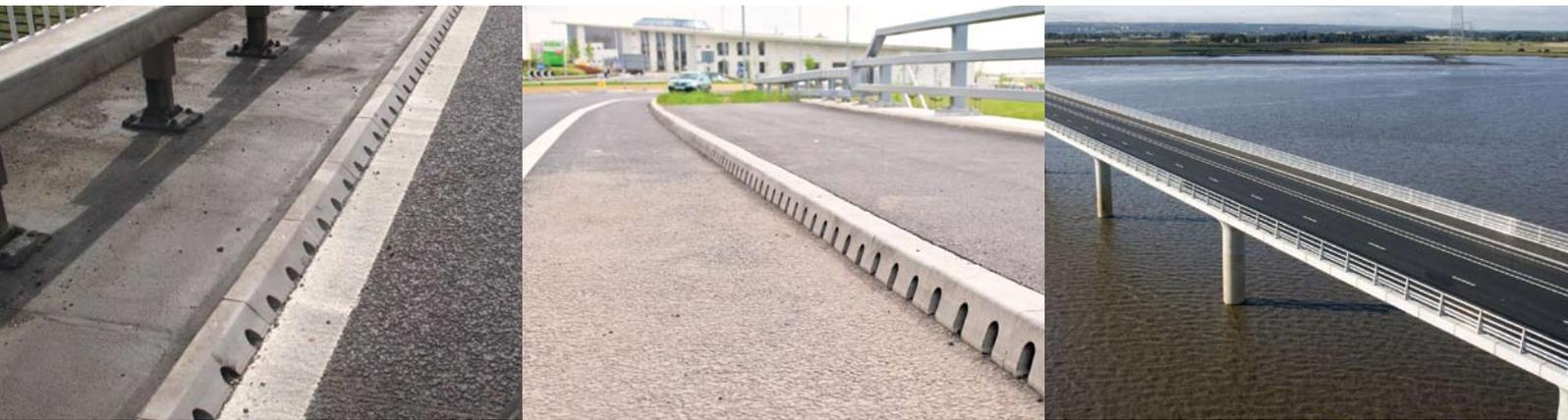
The product is available as 150mm, 220mm and 310mm wide with various depths depending on the Kerb Profile required (75mm, 100mm or 125mm splay or HB).
